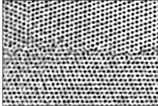
Figure 6.19: A TEM-image of Al (courtesy of the National Center for Electron Microscopy at the Lawrence Berkeley National Laboratory).
