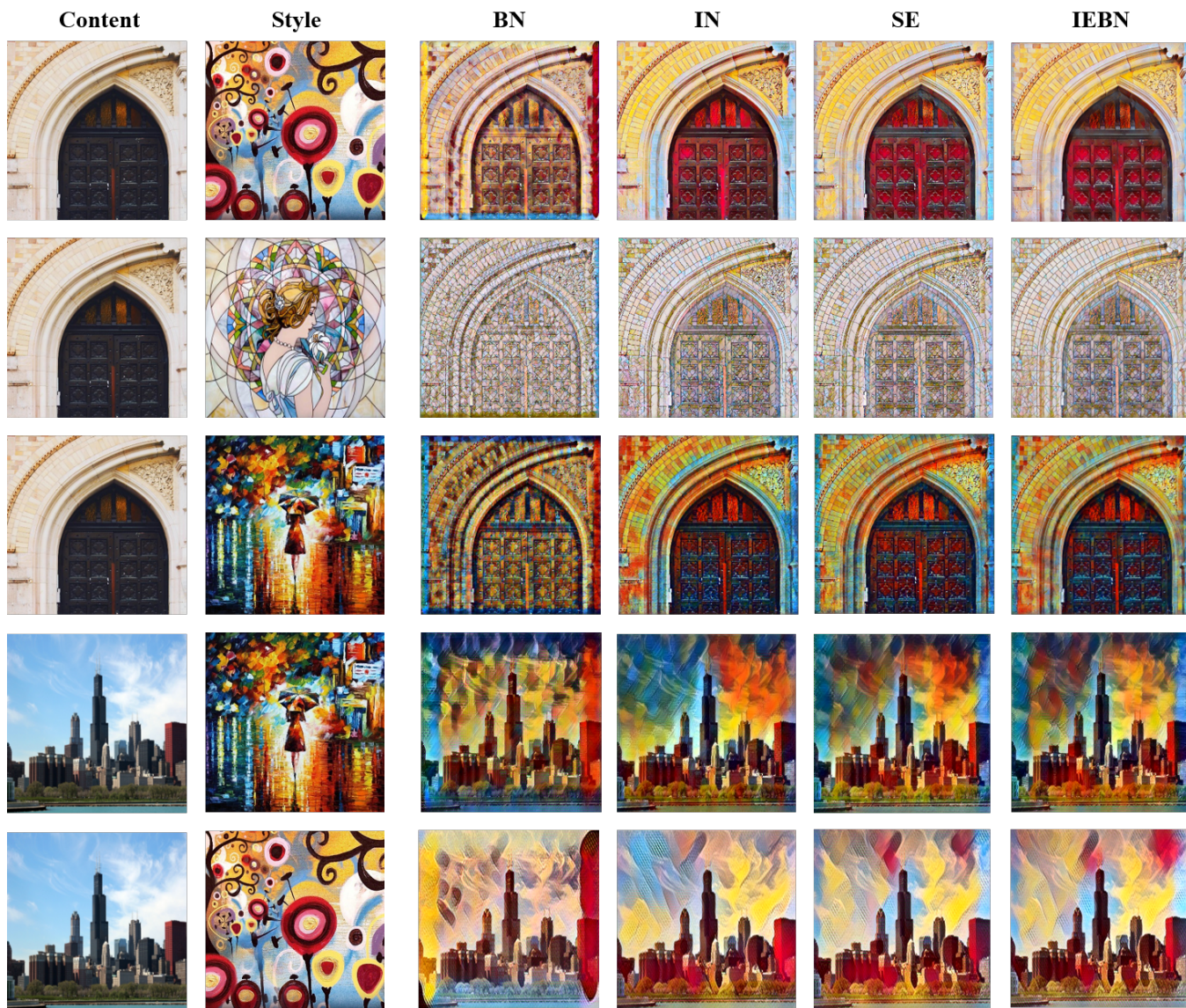
Figure 2: Stylization results obtained by applying style (second column) to content images (first column) with different normalization methods. Specially, “SE” means the transformation network with BN and SE module. The style of the generated images with BN appears more confused, but those with SE or IEBN are quite similar to IN visually.
