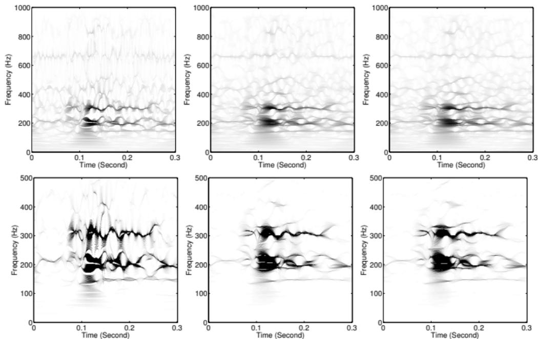
**Figure :** From left to right:  $s = 1$  (SSWT);  $s = 0.75$ ;  $s = 0.625$ . Top: whole domain. Bottom: low frequency part.
